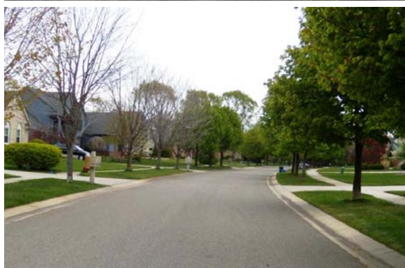
Varying street widths, building setbacks, and the presence of street trees and sidewalks can dramatically influence the speed of motorists
