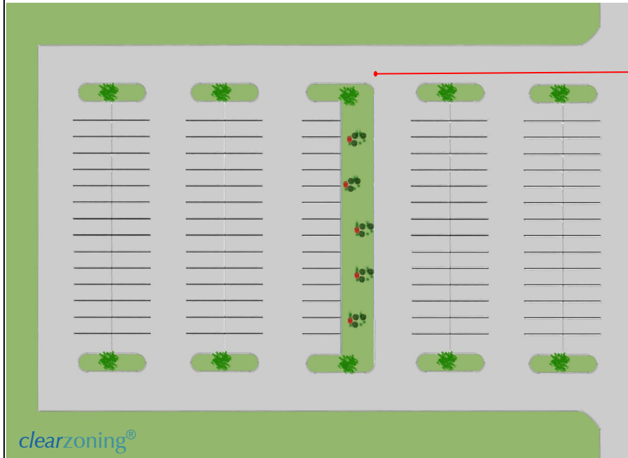
FIGURE 3.1.22.L.ii MINIMUM PARKING LOT LANDSCAPING REQUIRED
