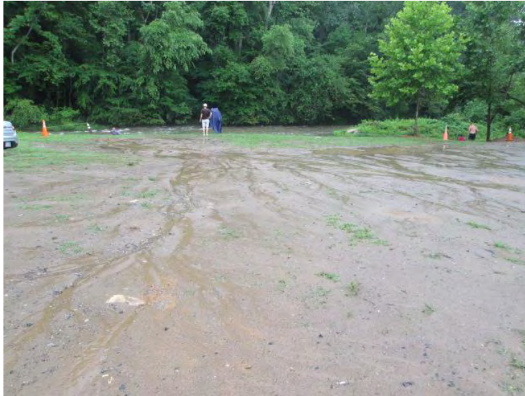
Photograph 24: View of Green River Cove Tubing parking area along the Green River near confluence with Gadd Creek at Site 2. Sedimentation from parking area discharges directly to the Green River.
