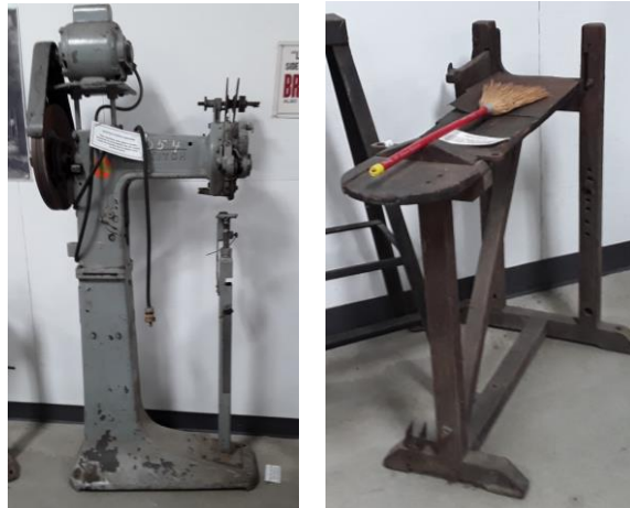
The Bostich staple machine (left) used to put metal cases on brooms and to staple wires on brooms and the broom repair bench (right) are part of the Lay Company display at the Jay County Historical Society. Photos courtesy of Kay Locker of the society.
