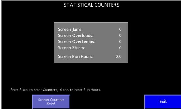
View the statistical counters. Press the button at the bottom left of the screen and follow the instructions to clear the counters and motor run time.
