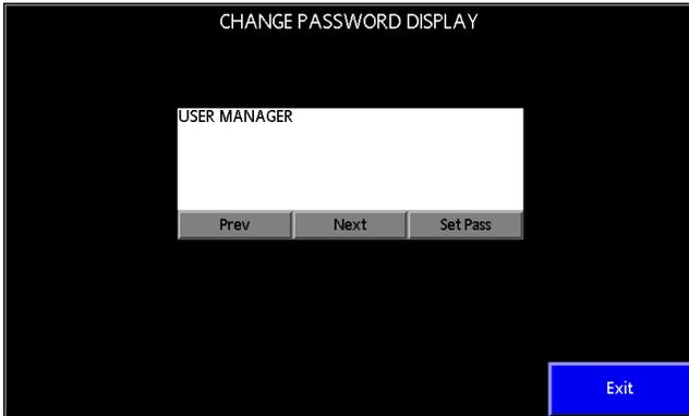
Press User Manager, enter a new four digit security password from the pop-up screen and press Set Pass to change the four digit security password.
