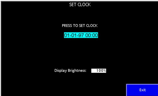
Press the set clock field and enter new values from the pop-up screen, then press Set Clock to change the PLC clock setting.
