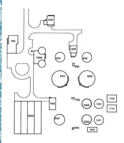
100 Administration Unit 1000 Final Clarifiers 200 Influent Pump Station 1100 Recirculation Pump Station 300 Grit Unit 1200 Digester Complex 400 Primary Clarifiers 1300 Sludge Beds 500 Control Structure No. 1 1400 Final Clarifier 600 Trickling Filters 1401 Final Clarifier 1700 AS Blower Building 700 Control Structure No. 2 800 Intermediate Clarifier 1710 Activated Sledge Basin 900 Control Structure No. 3 1800 Ultraviolet Disinfection
