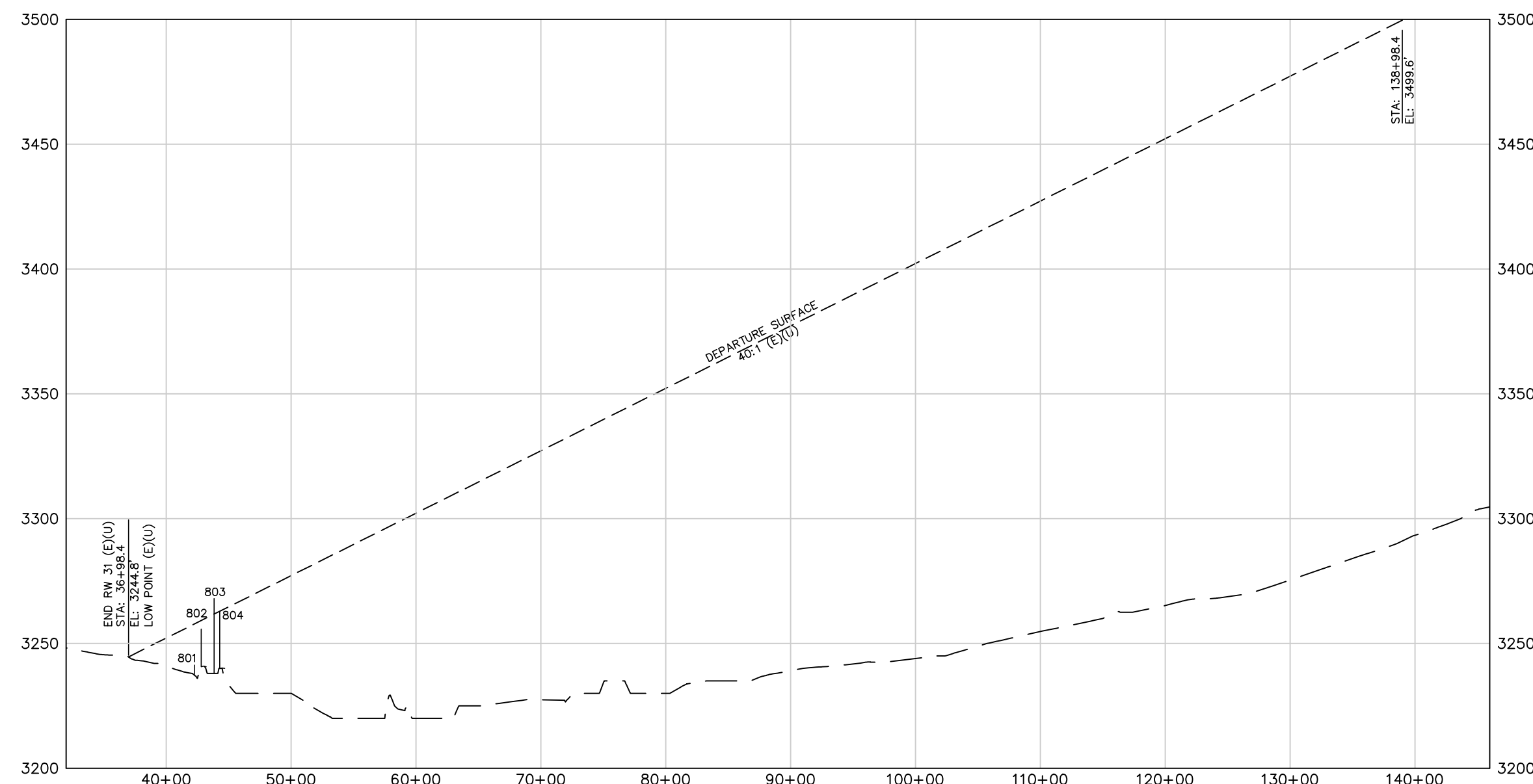
EXISTING AND ULTIMATE RUNWAY 31 DEPARTURE SURFACE PROFILE HORIZONTAL SCALE: 1"=1000' VERTICAL SCALE: 1"=50'
