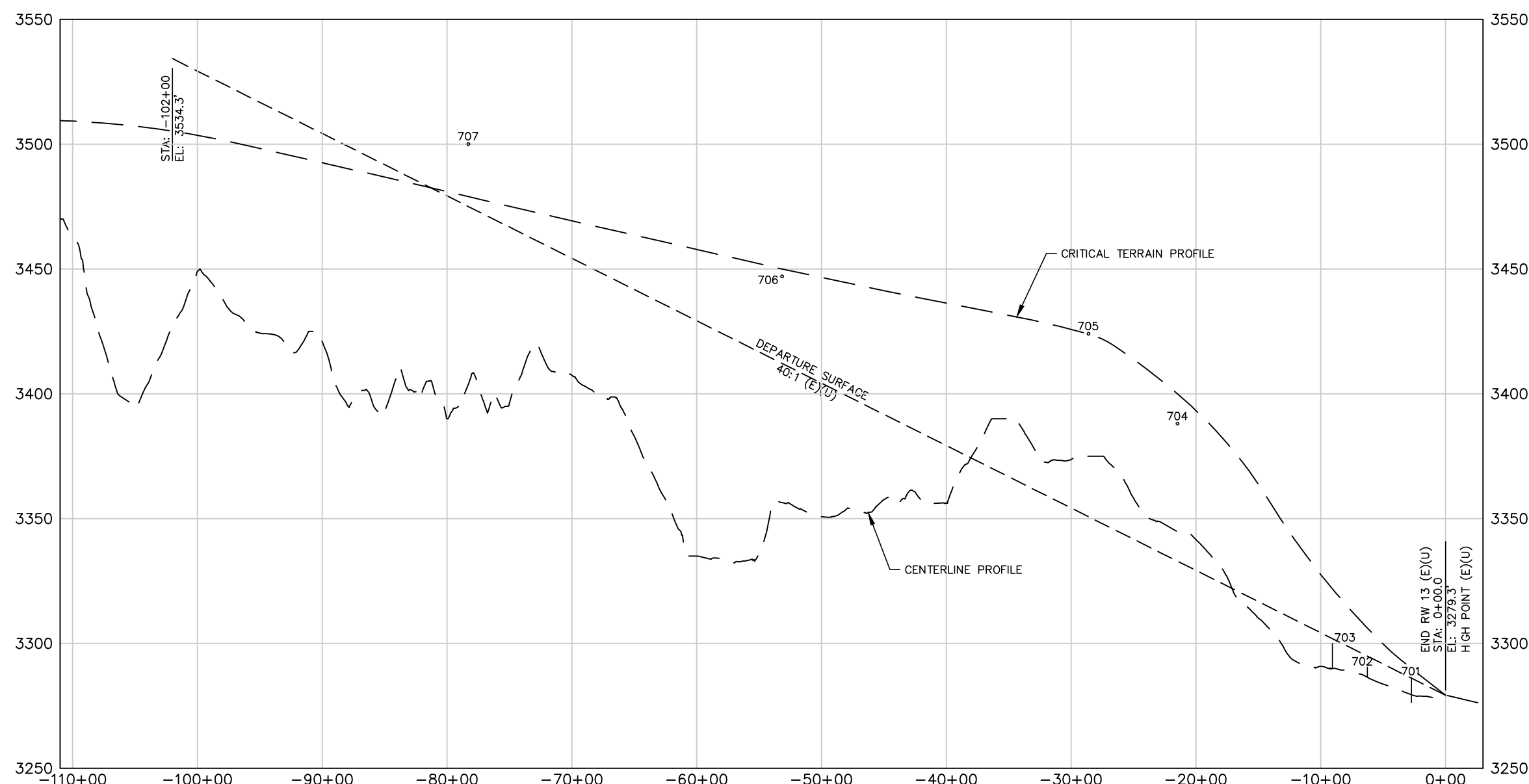
EXISTING AND ULTIMATE RUNWAY 13 DEPARTURE SURFACE PROFILE HORIZONTAL SCALE: 1"=1000' VERTICAL SCALE: 1"=50'
