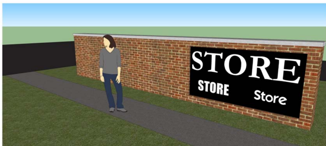
Monument Signs - the total area of the sign and support shall be no more than four times the sign surface display area. In this example, a 32 square foot sign surface display (area in black with white letters) is shown on a 128 square foot monument (5' x 25.6').
