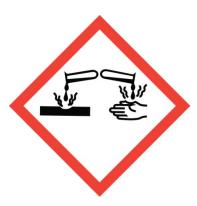
The red frame around the white diamond contains an image of two test tubes. One tube pours dripping liquid onto a solid black line, and the other tube drips liquid onto a hand. Both the solid line and hand image are eaten away where the liquids splash, emitting fumes. This symbol indicates:
