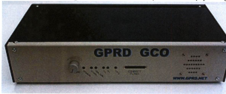
Typical Ground Communication Outlet (GCO) equipment
